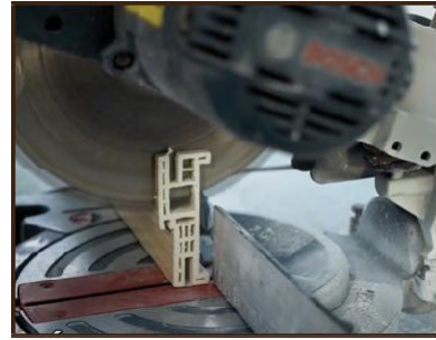
Step 2: Cut the vertical frame edges as the technique drawing.
